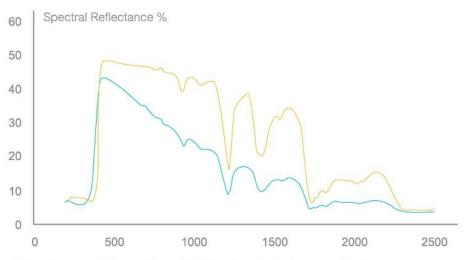
Yellow line stands for cooling turf / Blue line stands for normal turf
